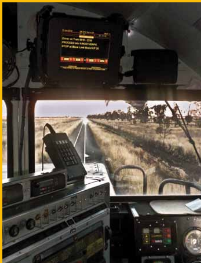
Driver's view: Monitor showing current authority, key pad, microphone and the track ahead. ARHSnsw Railway Resource Centre
